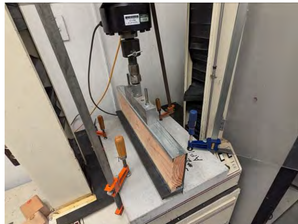
Photo 12: Transverse-Out Test Setup
