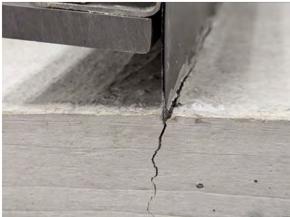
Photo 17: Failure of Transverse-Outward Tests
