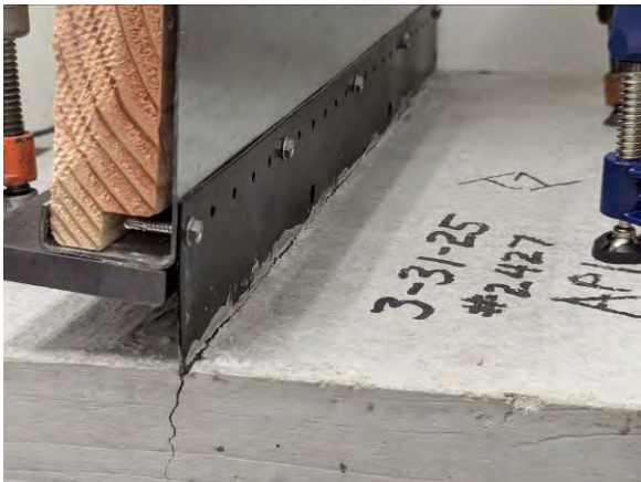
Photo 18: Failure of Transverse-Outward Tests
