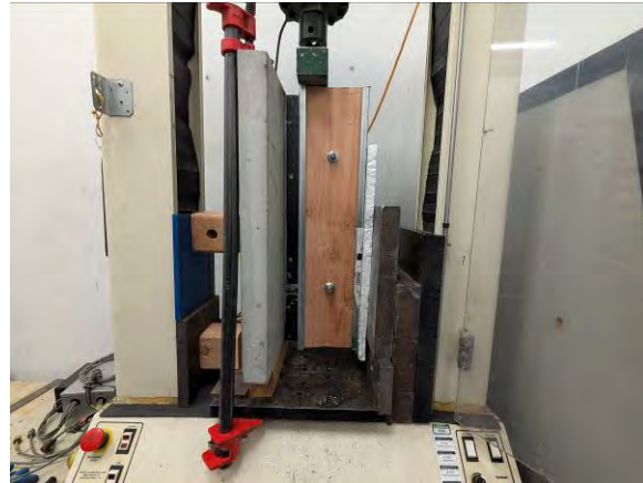
Photo 8: In-Plane Vertical Shear Test Setup
