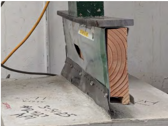
Photo 16: Failure of Transverse-Inward Tests
