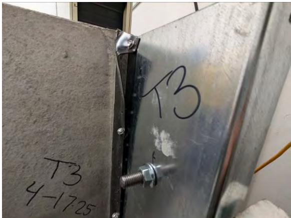
Photo 15: Failure of Test 3 Vertical In-Plane Shear
