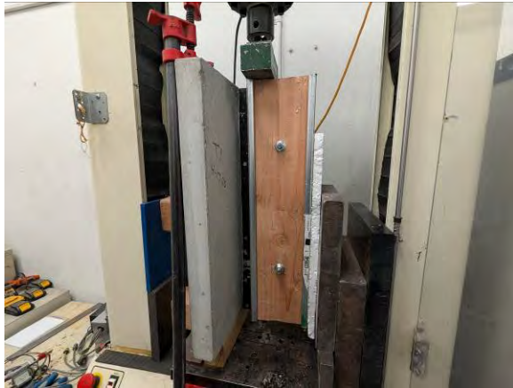
Photo 7: In-Plane Vertical Shear Test Setup
