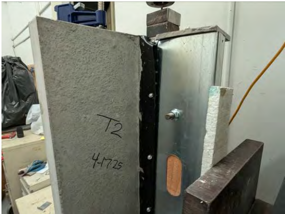
Photo 14: Failure of Test 2 Vertical In-Plane Shear
