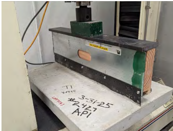
Photo 9: Transverse-In Test Setup
