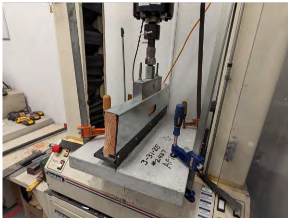
Photo 11: Transverse-Out Test Setup
