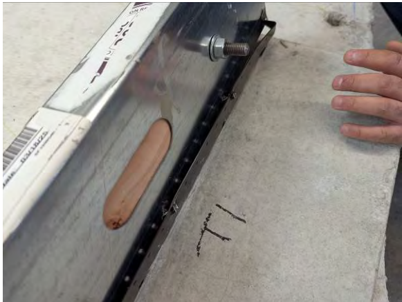
Photo 13: Failure of Test 1 Vertical In-Plane Shear
